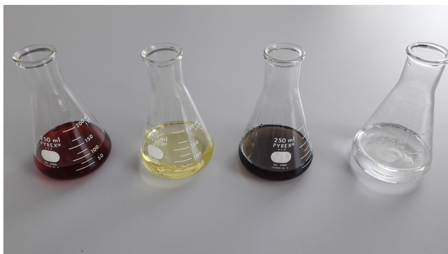
Figure 4 - from left to right: solutions of \text{KIO}_3 after the addition of \text{KI} and \text{HCl} - solution immediately before the endpoint - solution after the addition of starch - end of titration
