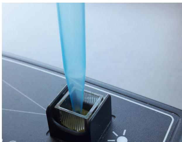
**Figure 1** - adding bleach to cuvette
