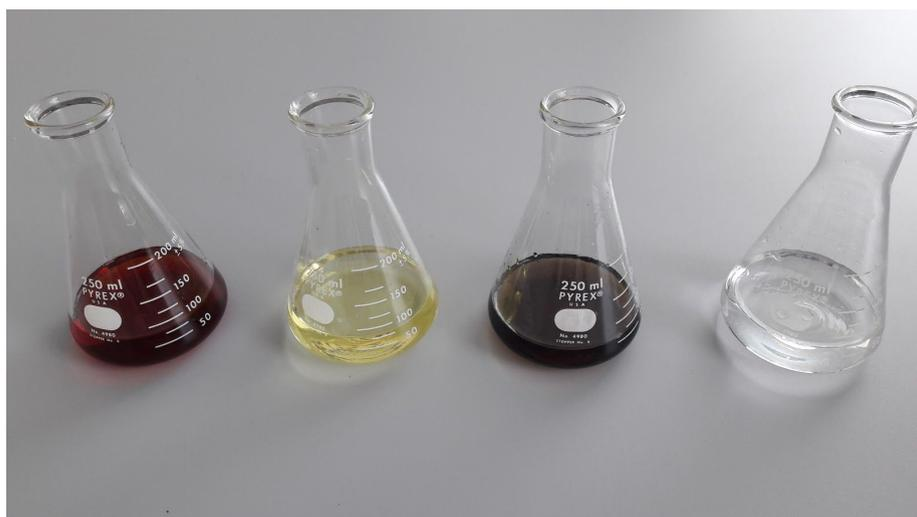
**Figure 4** - from left to right: solutions of  $\text{KIO}_3$  after the addition of KI and HCl - solution immediately before the endpoint - solution after the addition of starch - end of titration
