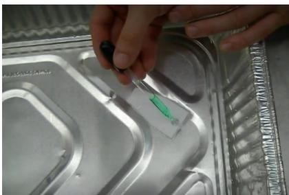
The soap boat experiment makes use of the Marangoni Effect, the tendency of material to move from a region of low surface tension to a region of high surface tension. Because detergent has a lower surface tension than water, when a drop of detergent is added to the fuel reservoir in the boat, the surrounding water “pulls” the soap out of the reservoir. The flow of soap out of the reservoir provides thrust to push the boat forward.
