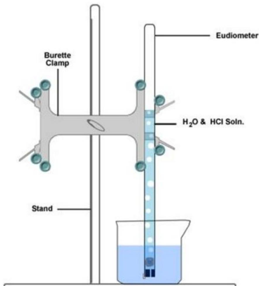
Work with a partner. A concentrated solution of HCl is going to react with a small piece of magnesium ribbon. Your job is to accurately predict the level of gas when the experiment is over. You must provide three items.
