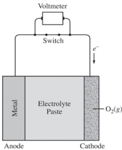
1. Metal-air cells are a relatively new type of portable energy source consisting of a metal anode, an alkaline electrolyte paste that contains water, and a porous cathode membrane that lets in oxygen from the air. A schematic of the cell is shown above. Reduction potentials for the cathode and three possible metal anodes are given in the table below.
