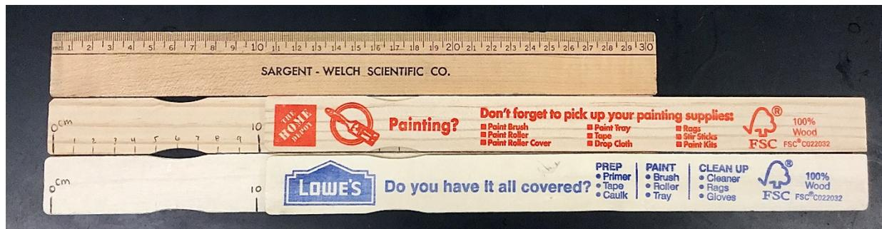
**Figure 1:** Note the different amount of markings on each of the rulers used for measuring in this lab. The Sargent-Welch ruler also uses cm.
