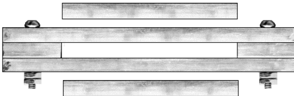
Figure 10.3. Diagram of the center bars and body of the die (actual size) described in Demonstration 10.1. All components are made out of 1/4-inch square stainless steel rods. (The center bars are of the correct length to just fit in the gap in the center of the body of the die.) Holes are drilled through the six bars forming the body, and small nuts and bolts are used to secure the pieces as shown. The body of the die is placed on a piece of cardboard that has a hole cut in it that is the shape of one of the center bars. A center bar is pushed through the hole in the die body and into the hole in the cardboard. In this way, the body of the die is held above the center bar. The cardboard and center bar will rest on the counter (or, on the base of the press). The powder may then be placed on the center bar. The second center bar is then placed on top of the powder. When the press is used, the powder is squeezed between the two center bars. After releasing the pressure, the pressed sample may be removed from the die by carefully removing the top center bar and loosening the bolts.
