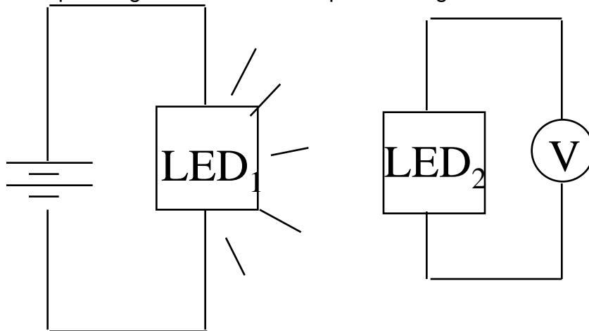
The red LED causes photovoltage in the green LED
